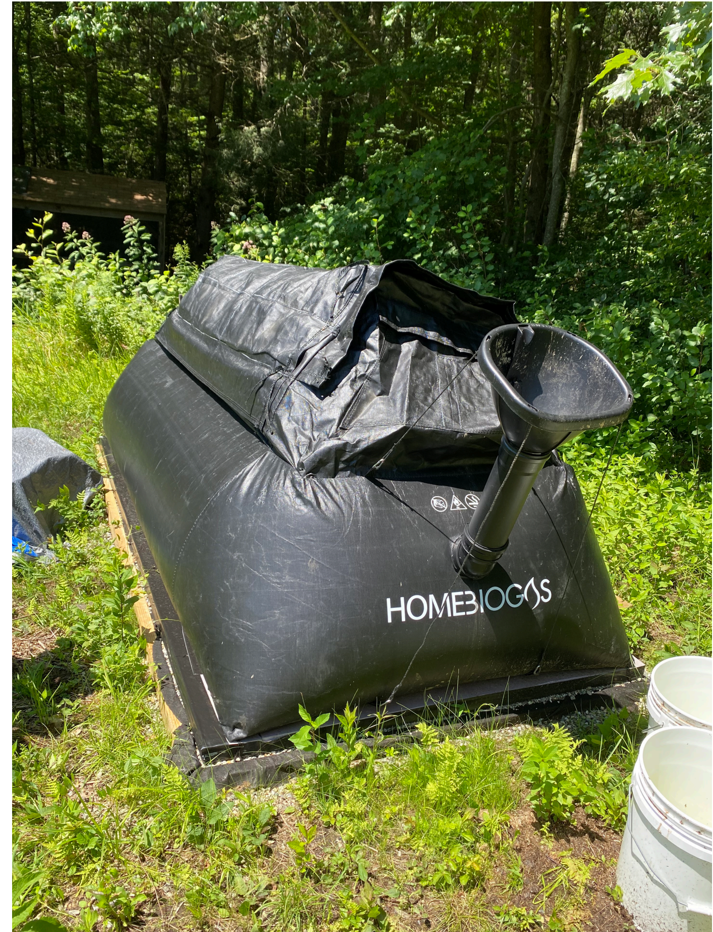
Commercial Biogas Bag System, small farm digester, 2.5 cubic meters
