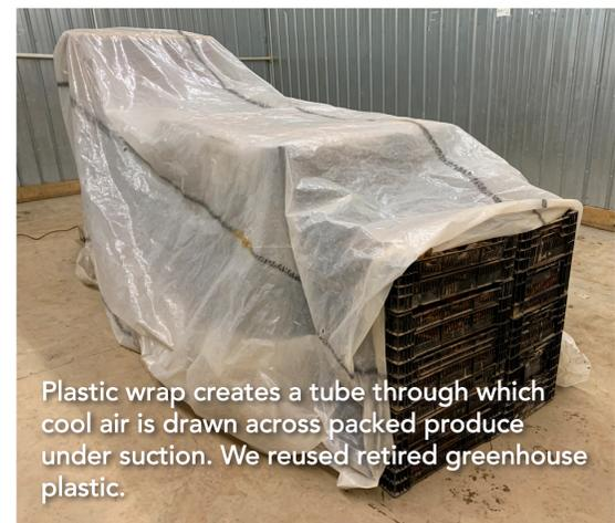
Plastic wrap creates a tube through which cool air is drawn across packed produce under suction. We reused retired greenhouse plastic.
