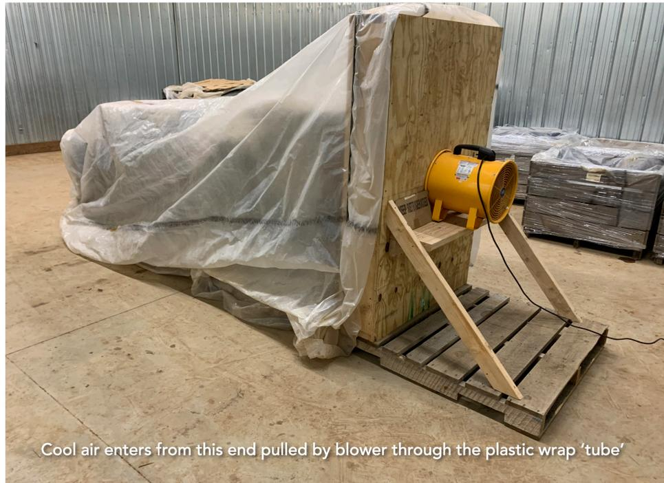
Cool air enters from this end pulled by blower through the plastic wrap 'tube'
