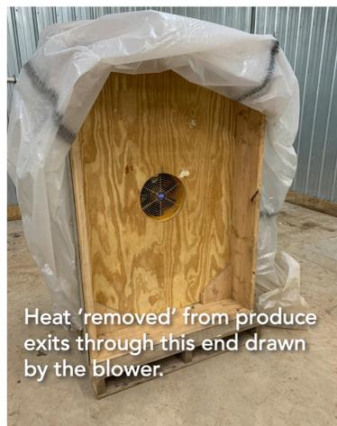
Heat 'removed' from produce exits through this end drawn by the blower.
